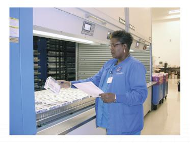
Upon distribution, the VLM delivers the item to the operator for picking. The item is placed in a bin and sent to verification where it is verified, packed and sent to shipping. The package is verified once more and shipped based on criteria such as if the items are frozen or room temperature.
